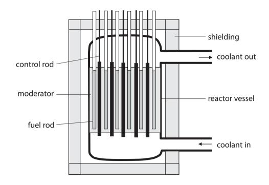
(a) Draw a line linking each part of the reactor with its main function.
